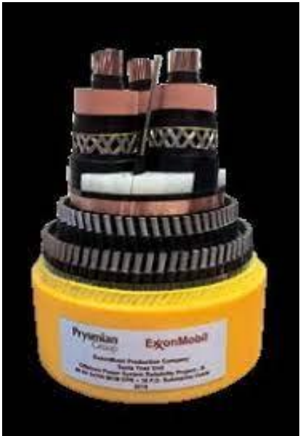
Typical 66 kV cable design for offshore wind
